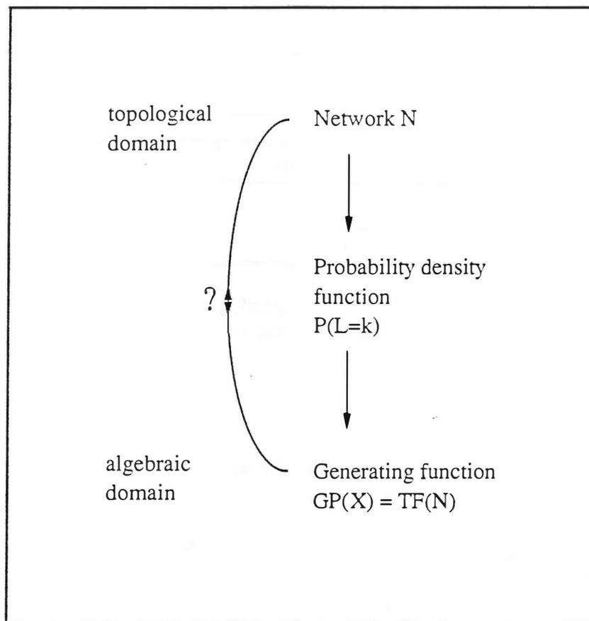
Fig. 2. A conceptual overview of the model. The by-pass is represented by the question mark.
