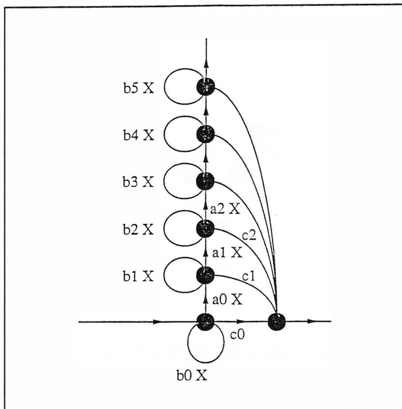
Fig. 8. An example of a universal network, capable of modelling any arbitrary duration distribution.
