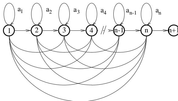
Figure 4.6. A general left-to-right HMM with  $n$  selfloops and all possible skips.
