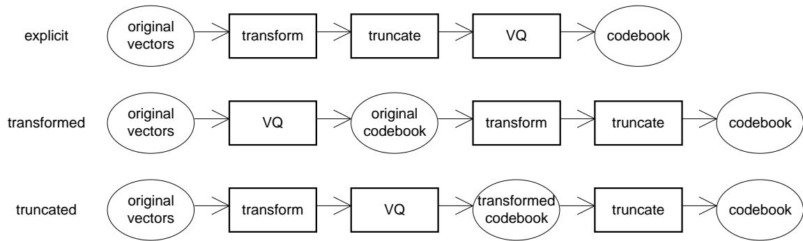
Figure 3.1 Three approaches to obtain transformed and truncated codebooks. Rectangles indicate processes, and ellipses are objects.
