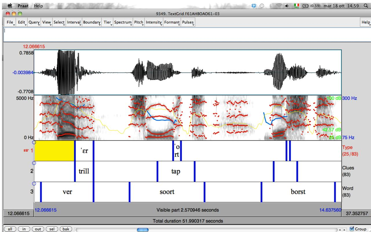
**Fig. 8.2.** A picture of the *Praat* textgrid window during the segmentation stage: adding borders and labelling intervals. You can see the three windows: from top to bottom: the sound wave, the spectrogram and the three tiers. On the right side you can see the names of the three tiers. No cues were found for the r-sound in *borst* ‘chest’, so the interval has been left unwritten for the following automatic analysis.
