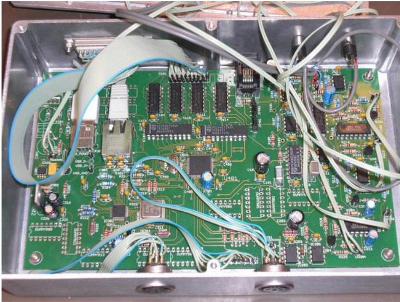
Figure 5: EventBox with internal electronics
