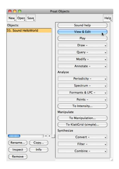
In the menus that appear to the right of the object list you see all the things you can do to the Sound: playing, drawing, querying, modifying, annotating, analysing, manipulating, converting, filtering, and combining it with other Sounds (if these are selected as well). The most "attractive" button, however, says **View & Edit**, and if you click it (or just press the Enter key), the selected Sound pops up in a new Sound window:
