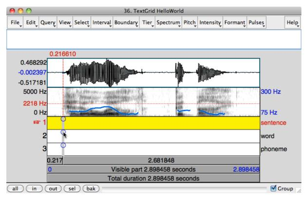
This TextGrid window shows three things: at the bottom, the contents of the TextGrid, which is initially just three empty tiers; at the top, the waveform of a copy of the Sound; in the middle, some analyses (in the figure, a spectrogram and a pitch contour) of this copy of the Sound.
