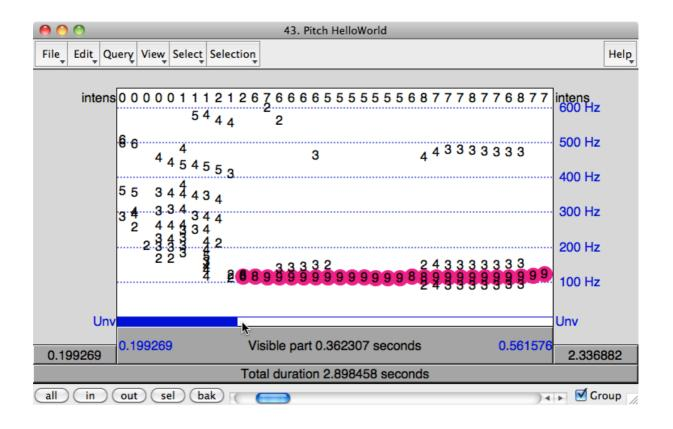
This Pitch window contains numbers between 1 and 9 to depict the quality of separate pitch candidates, red dots to mark the pitch candidates that are in the current optimal path, and a blue "unvoiced" bar at the bottom. You can click on the numbers and on the unvoiced bar to modify the pitch curve. Please note that the representation of the Pitch object in this window is quite different from its representation in the Picture window above.
